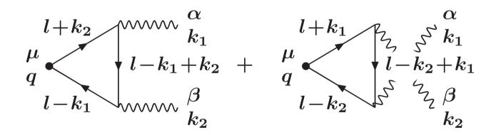
Note that the second diagram is identical to the first one but with crossed external photons with  $(\alpha, k_1) \leftrightarrow (\beta, k_2)$ .
