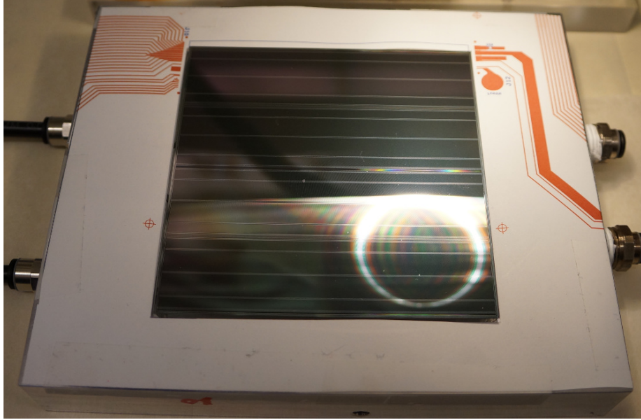
Figure B.4: Sensor placed on vacuum jig.
