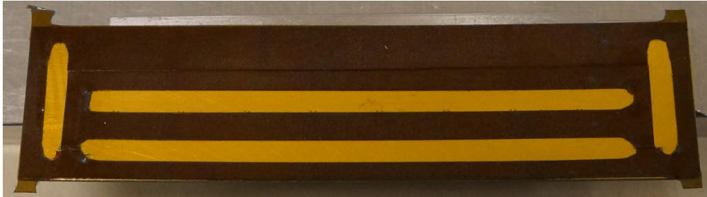
Figure B.2: Mask for the glue attached to back of the hybrid. The wings in the four corners have to be removed. The frame on the border of the hybrid will stay. The inner part will be removed after the glue is applied.
