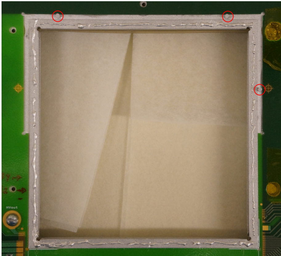
Figure B.7: Silver epoxy applied on the HV frame to make contact between the back plane of the sensor and the bias voltage.
