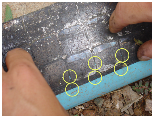
Figure 8: The location of several holes in the iron sheet due to corrosion.
