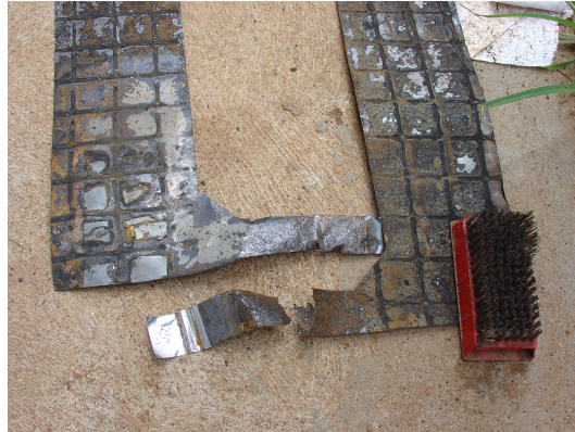
Figure 7: Ripped electrode due to corrosion.
