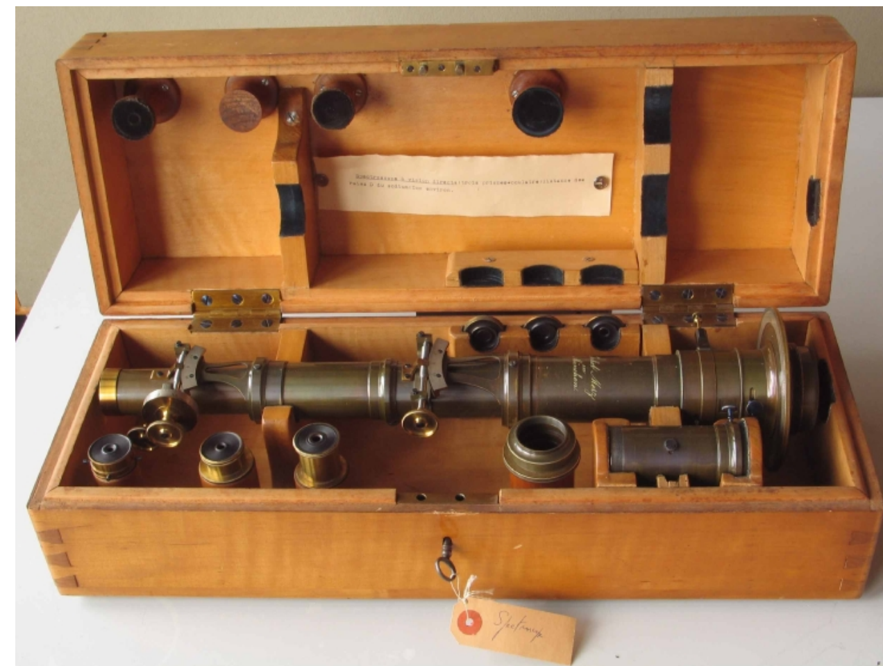
Direct-vision spectroscope 3 trains of 3 prisms Jakob Merz (München) (l = 480 mm)
