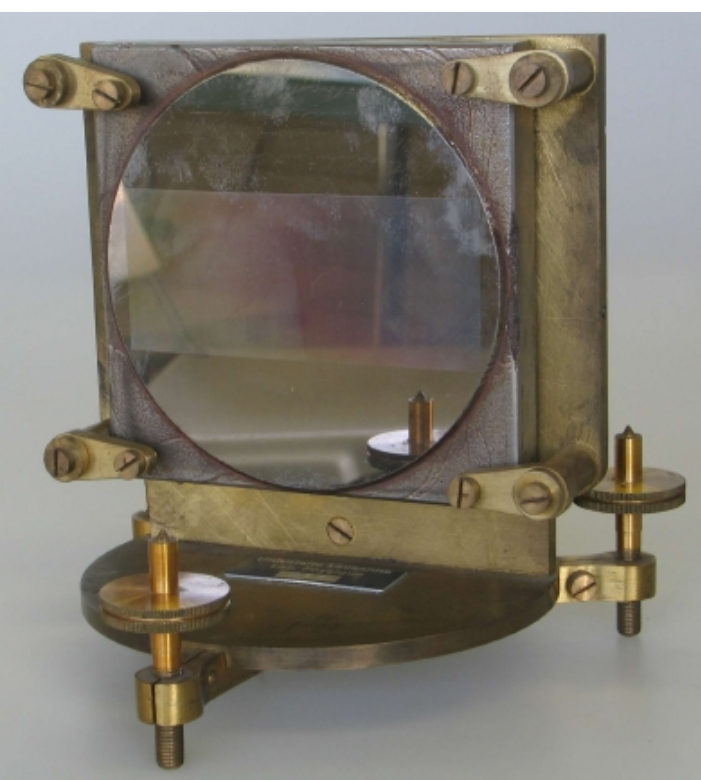
Metal diffraction grating Rowland (Baltimore), 1888 14'438 lines/inch ( \varnothing 100 mm)
