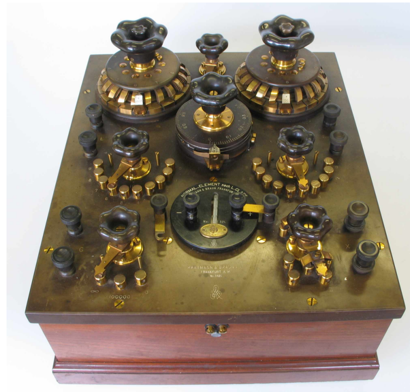
Hartmann & Braun (Frankfurt a. M.), 1900-1908 The reference is still a Clark element (width 370 mm)
