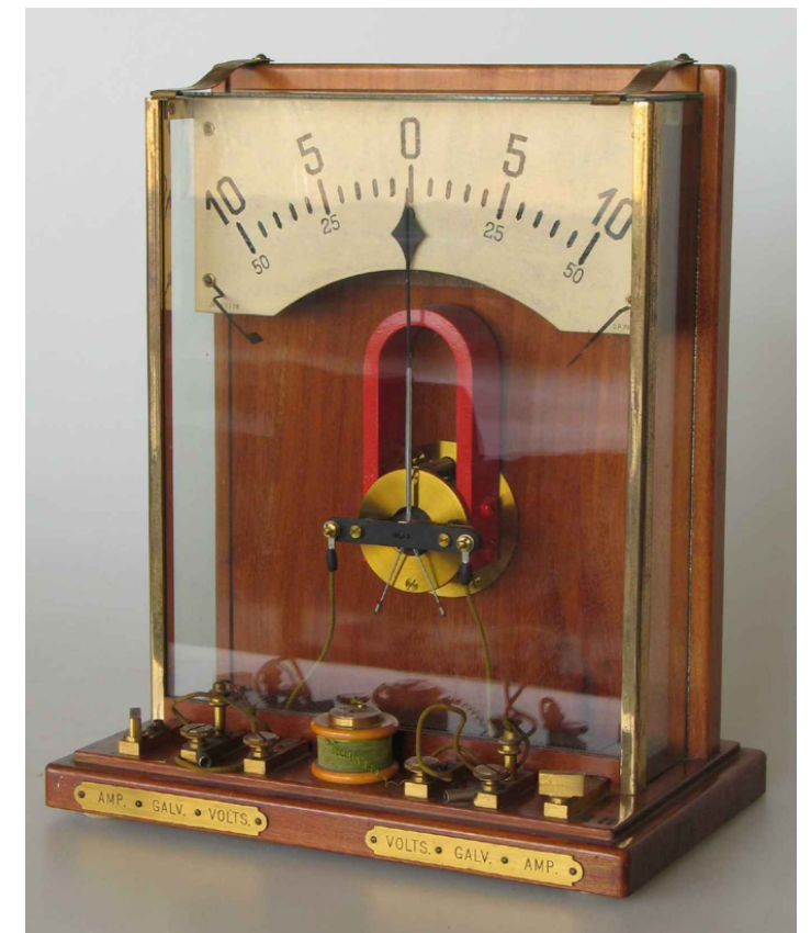
Demonstration moving coil V-/A-meter Hartmann & Braun (Frankfurt a.M.), after 1897 (h = 340mm)
