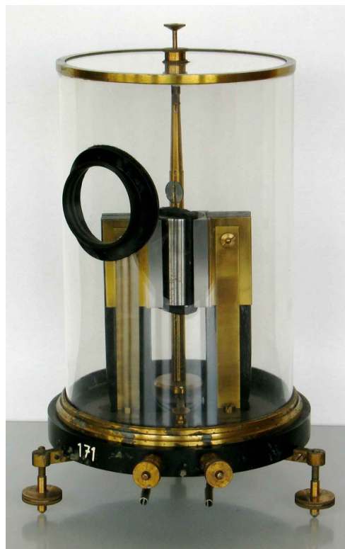
Moving coil galvanometer J. Carpentier (Paris), after 1889 (h = 310 mm)
