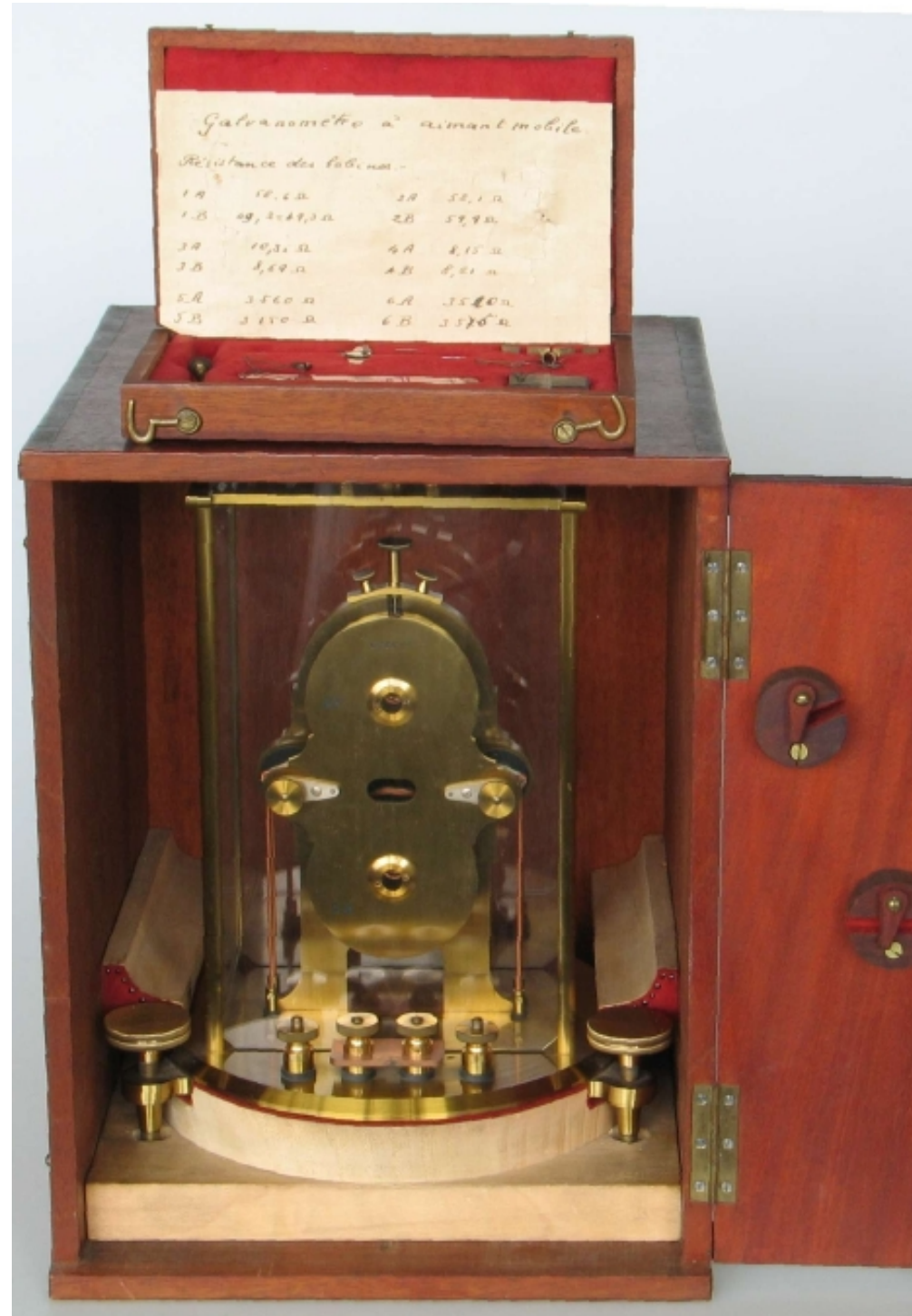
Astatic galvanometer and accessories At. Ruhmkorff – J. Carpentier (Paris) (box height 230 mm) On the top, box with magnetic needles and suspension threads Compensation magnets lost
