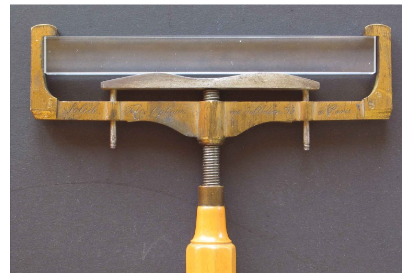
Stress induced birefringence Soleil Fils (Paris) (l = 158 mm)
