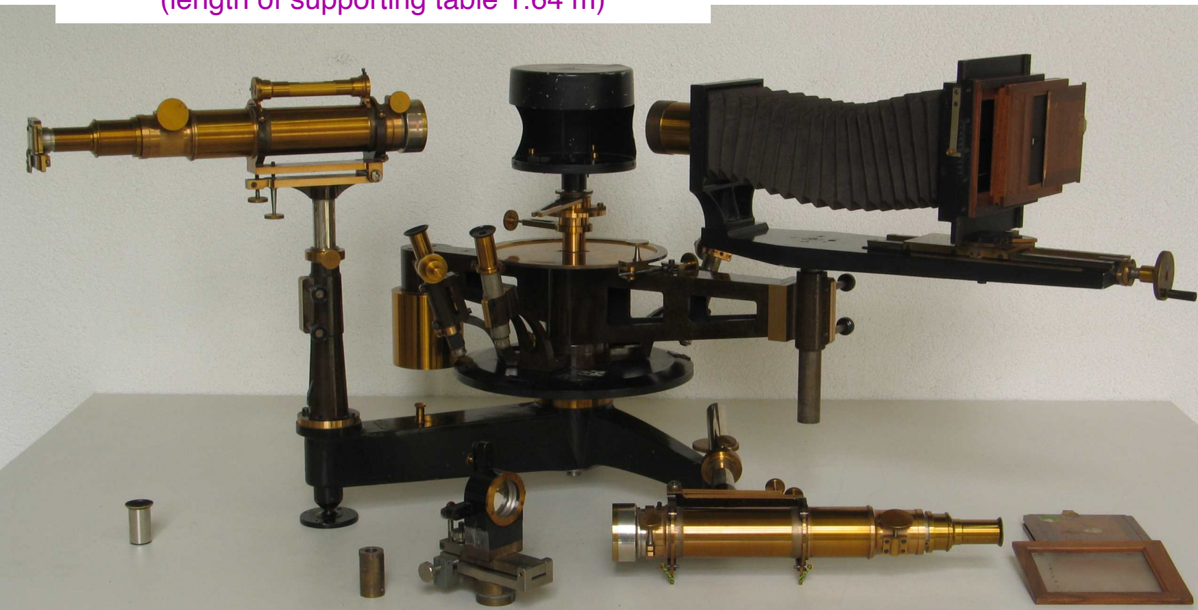
Two-arm spectroscope / spectrograph SIP (Geneva), after 1913 (length of supporting table 1.64 m)
