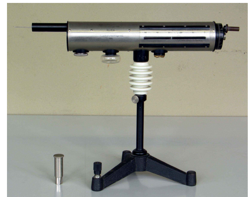
Wulf's coaxial capacitor Leybold (Köln), after 1925 (l = 390 mm)
