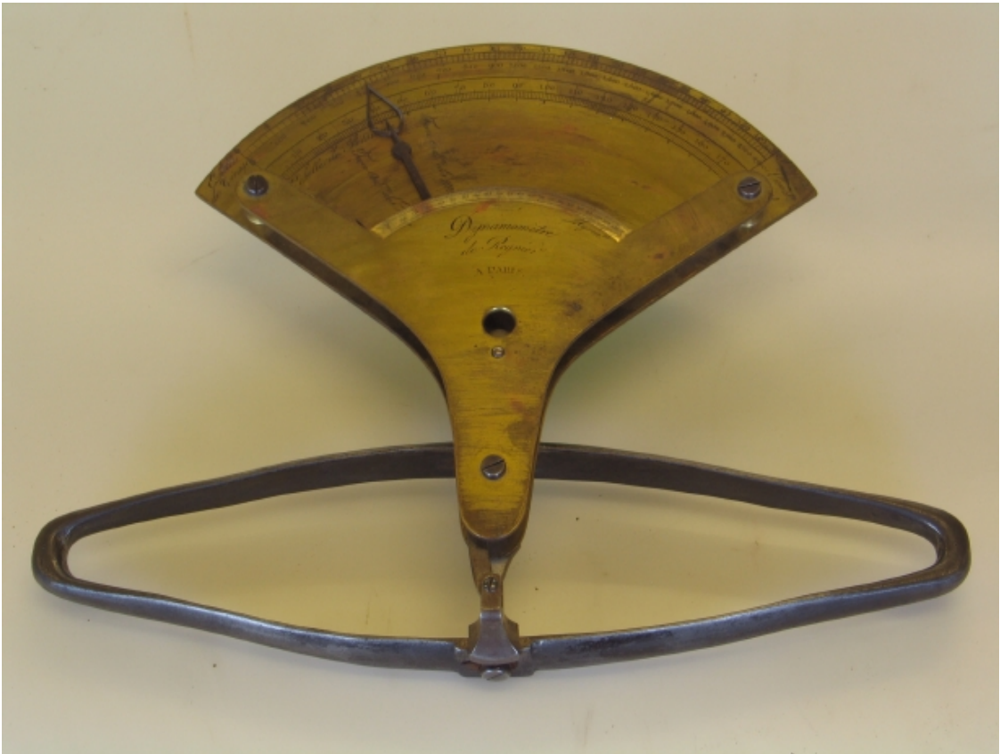
Regnier's dynamometer Invented 1798 (Paris), Tested in Lausanne in 1841 (spring length 310 mm)
