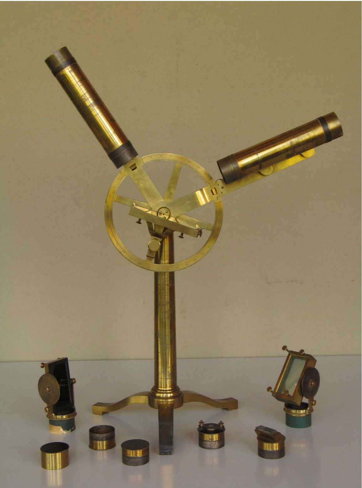
Apparatus to demonstrate polarisation phenomena, including black glass mirrors, pile of glass slides, parallelepipedic prism, etc. Probably French, undated (circle Ø 200 mm)
