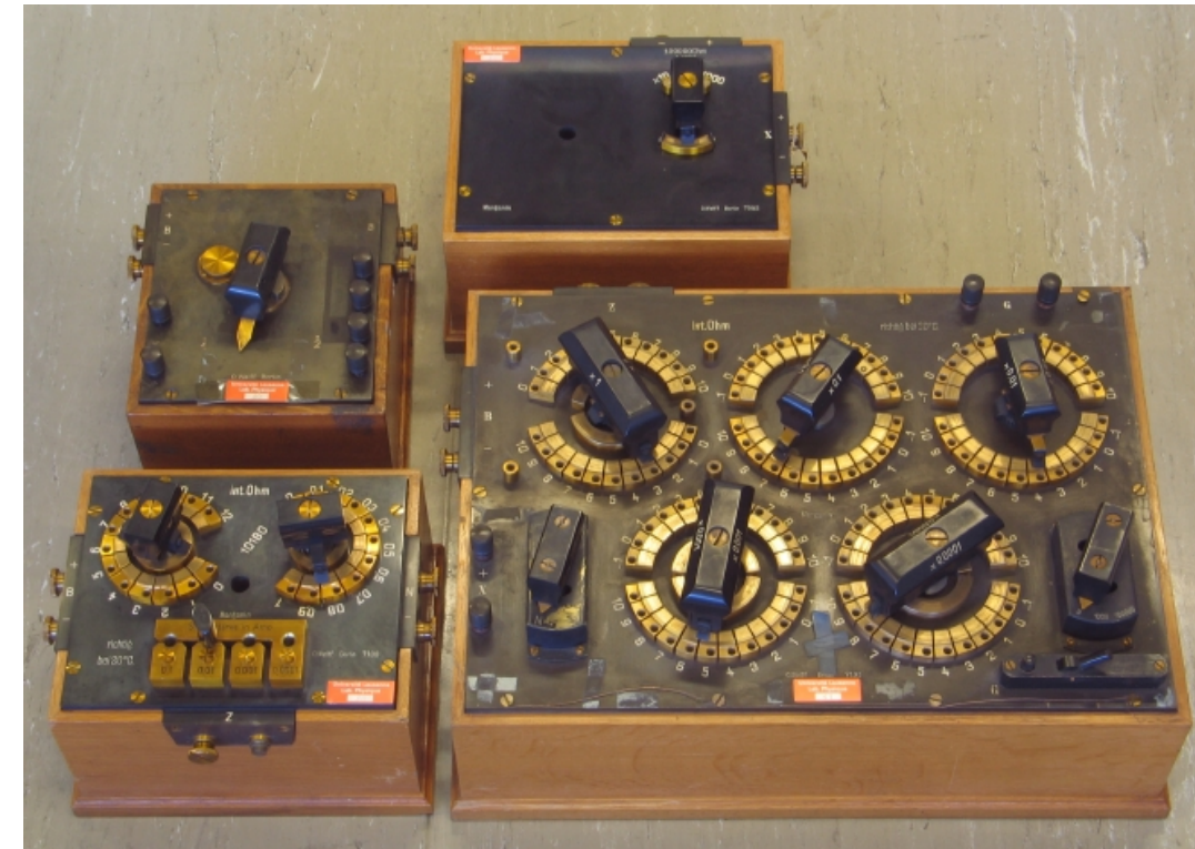
« Thermokraftfrei » after Diesselhorst, with Auxiliary Resistors Box, Switch and “Multiplier” O. Wolff (Berlin), after 1908 Pot. length 450 mm
