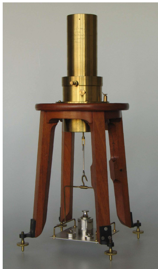
Exner electroscope with Elster-Geitel readout Spindler & Hoyer (Göttingen) (Ø 83 mm)
