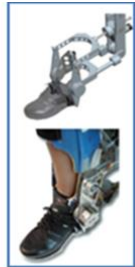
(b) Realization of the leg orthosis.
