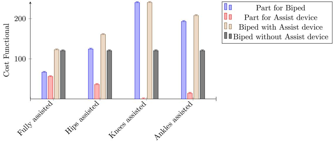
Figure 3: The torques of the biped and walking assist device are minimized: Histogram as a function of different distributions for the torques.
