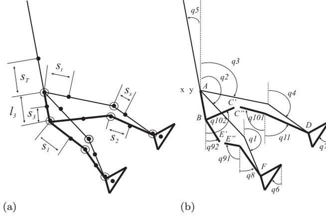
Figure 1: Planar biped with its walking assist device in bold line.
