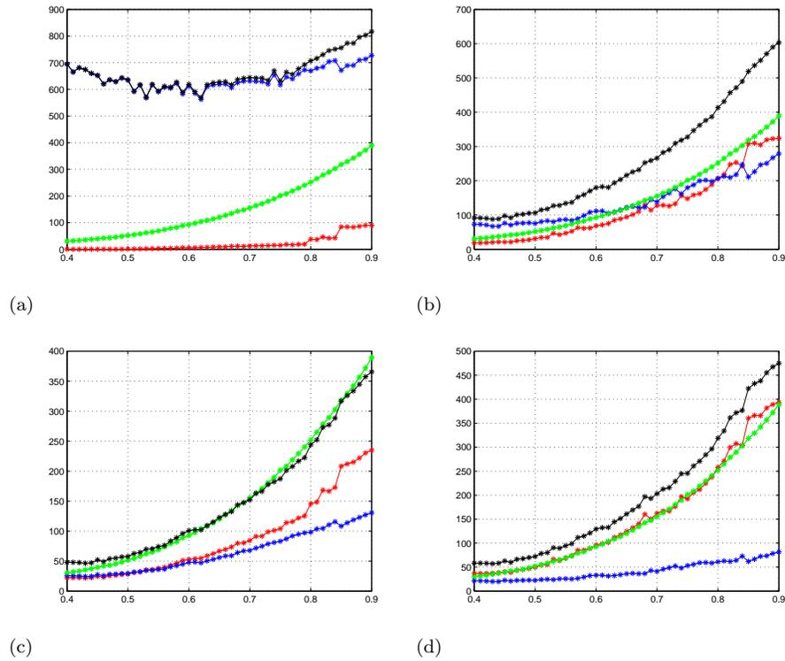
Figure 4: Torque cost as function of the velocities: Biped without assistance (green), Part for Assist device (blue), Part for Biped (red), Addition of the biped and assist device parts (black). (a) fully actuated, criterion  $C_{1k}$ ; (b) fully actuated, criterion  $C_{2k}$ ; (c) assistance in the hips only, criterion  $C_{1k}$ ; (d) assistance in the hips only, criterion  $C_{2k}$
