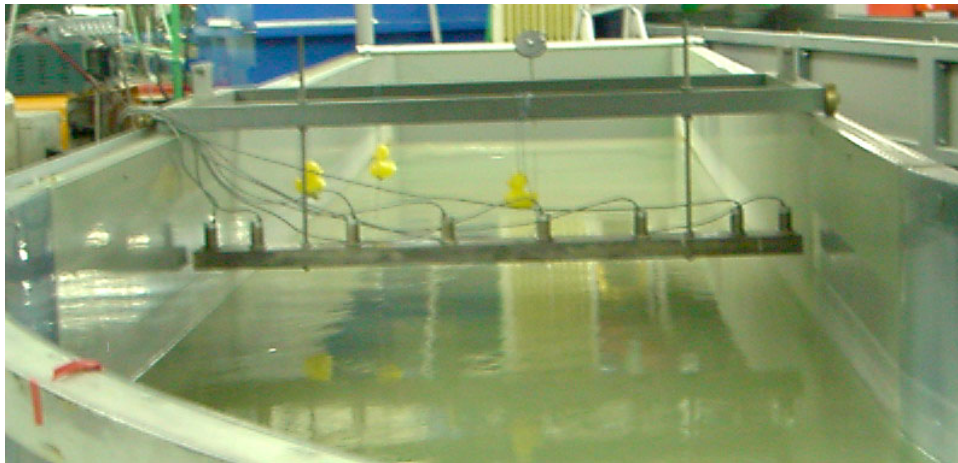
Fig. I.5: Acoustic limnimeters for measuring water-surface and bottom topography
