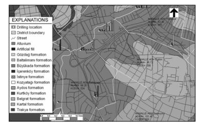
In the alluvial deposits of the studied area, the changing of standard penetration test (SPT) results with respect to depth is represented by bar graphs (as illustrated by figure 4).
