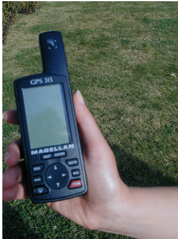
Figure 2 Low cost handheld type GPS is used for this study.
