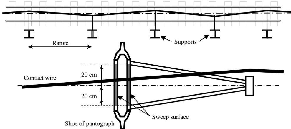
Fig. 11.14 Periodical misalignment on a right line.
