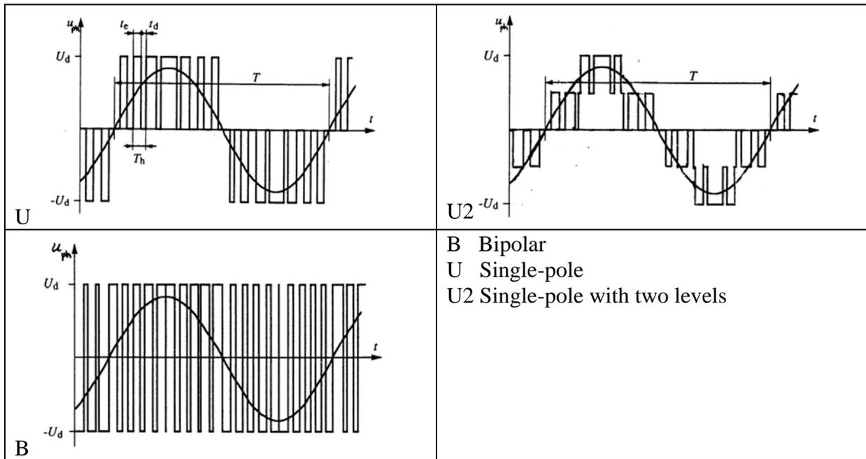
Fig. 4.168 Inverter arm-control.
