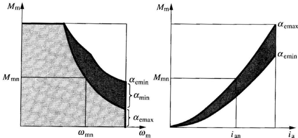
Fig. 4.143 Characteristics in traction with field weakening.
