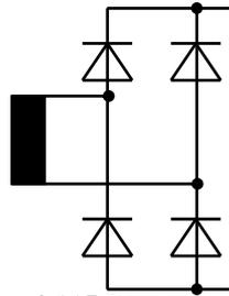
Fig. 4.115 Diode bridge.
