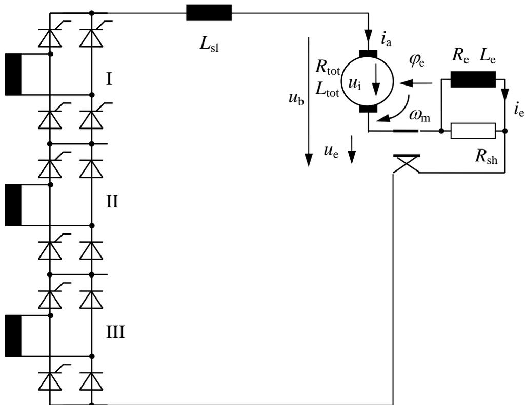
Fig. 4.139 A Three bridges in cascade. (SJ : Rc 1).
