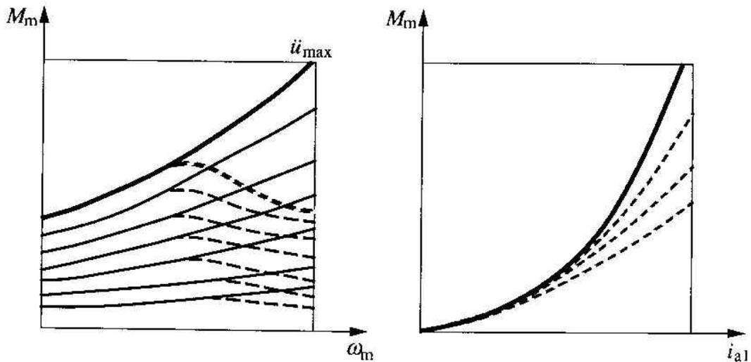
Fig. 4.61 Regenerative braking with separate excitation: characteristics.
