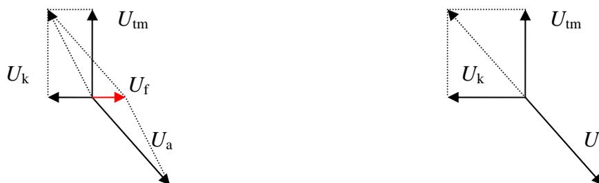
Fig. 4.40 Commutation in single-phase motor at low or nominal speed.
