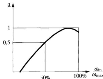
Fig. 4.62 Power ratio for braking with excitation motor.
