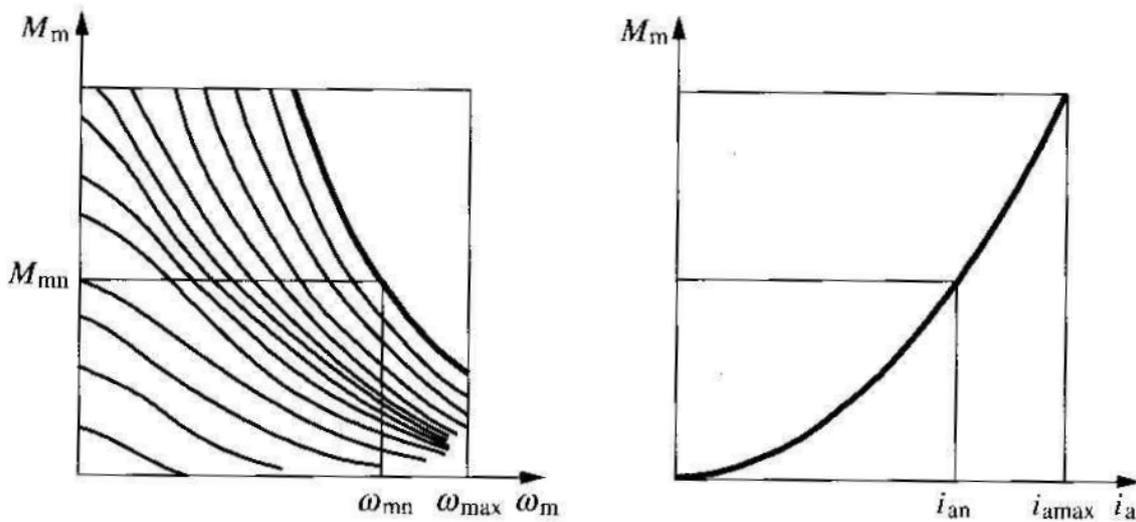
Fig. 4.44 Direct motor in traction: torque characteristics versus current and speed.
