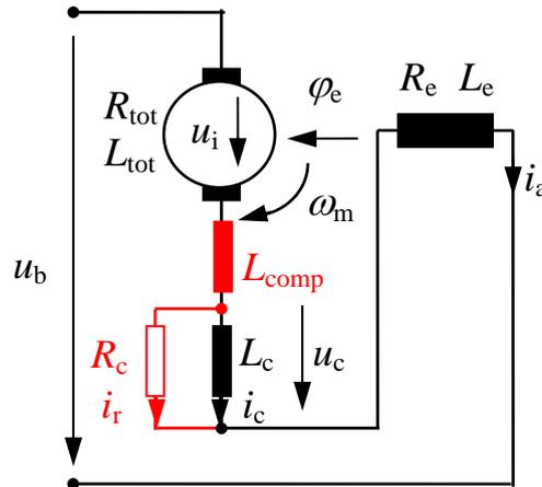
Fig. 4.37 Windings in single-phase motor.
