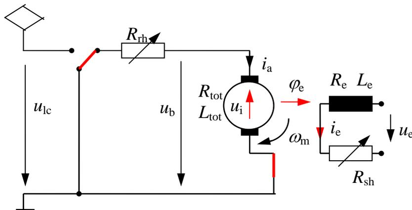
Fig. 4.13 DC-motor: rheostatic braking with separate excitation.
