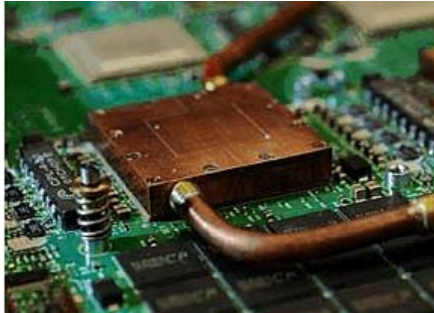
Integrated micro-channel cold plate in single chip
