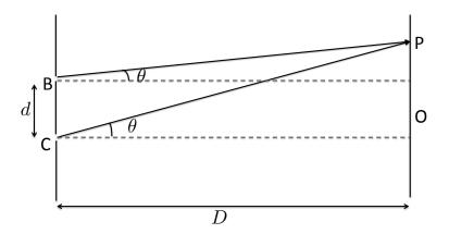
We assume that the waves diffracted by each slit have a spherical shape ( $\lambda$  the wavelength and  $\nu$  the frequency):
