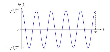
The receiver then processes the received signal R(t) through the matched filter  $h_j(t)$  to obtain  $(R \star h_j)(t)$ . This signal is sampled at time T to yield the value needed for the MAP decision.
