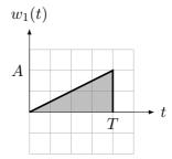
(a) Describe an ML receiver that decides which pulse was transmitted. The *n*-tuple former must contain a single causal matched filter. Finally, draw the matched filter impulse response.
