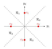
The distance between two adjacent codewords (say  $c_0$  and  $c_1$ ) is  $d = \sqrt{2\mathcal{E}}$  and the error probability of the receiver is
