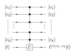
So U acts on the target bit if and only if all control bits are set to 1. By increasing the work space this gate can be represented by a concatenation of controlled-controlled-NOT and a controlled U. Indeed:
