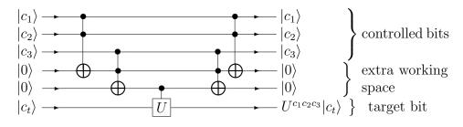
The controlled-controlled-NOT gate is also called Quantum Toffoli. Remarkably, it can be represented by one and two-bit quantum gates  $\{T, S, H, CNOT\}$ . Remember that classically this is not possible! The reader can check that
