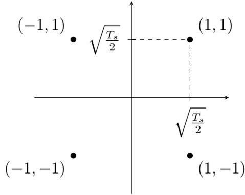
The mapping is such that neighboring points differ by one bit. This minimizes the bit-error probability since when we make an error chances are that we choose a neighbor of the correct symbol. Notice that we may decode each bit independently. In fact the first bit is decoded to a 1 iff the observation is to the right of the vertical axis and the second bit is 1 iff it is above the horizontal axis. The bit error probability is therefore
