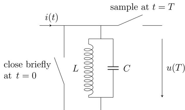
Since this circuit integrates and then dumps, it is called the *integrate-and-dump* circuit.
