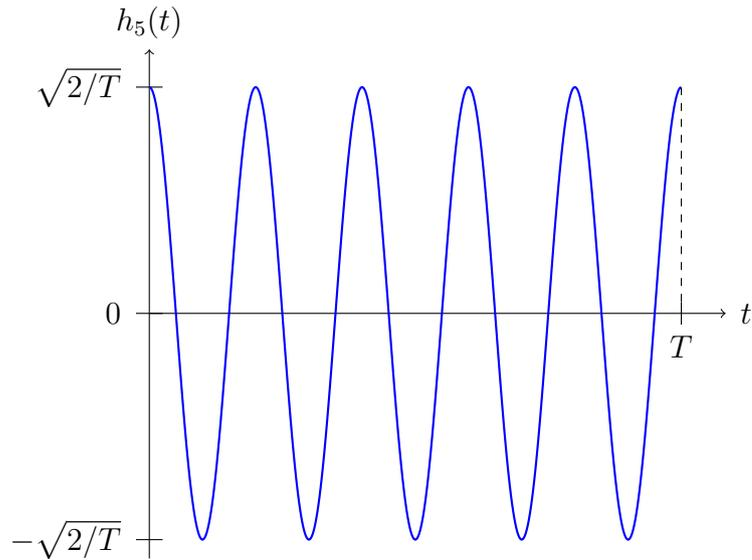
The receiver then processes the received signal  $R(t)$  through the matched filter  $h_j(t)$  to obtain  $(R * h_j)(t)$ . This signal is sampled at time  $T$  to yield the value needed for the MAP decision.
