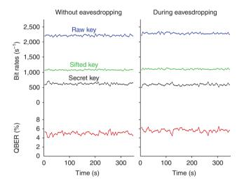
**Figure 3 | QKD performance with and without eavesdropping as measured by Alice and Bob.** Session without Eve in the fibre line (left). Eve installed (right). The traces in the top chart correspond to the raw key rate, sifted key rate and final secret key rate after error correction and privacy amplification<sup>18,20</sup>. The bottom chart shows the quantum bit error ratio (QBER).
