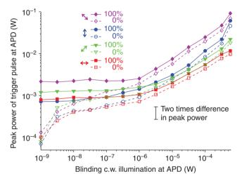
**Figure 4 | Click thresholds of the four detectors in Bob's PA versus blinding c.w.** power. The dashed curves show the highest peak pulse power at which the detector still never clicks. The solid curves show the lowest peak pulse power at which it always clicks. Between these two thresholds, click probability of each detector increases gradually. The detector recording photons of horizontal polarization (curves with squares) was the one tested in Figure 2.
