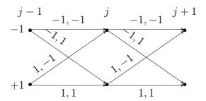
As the figure shows, the trellis has two states labeled with +1 and -1, respectively. The probability assigned to each of the two branches leaving any given state is  $\frac{1}{2}$ . The trellis is also labeled with the output produced when a branch is traversed and with the trellis depths j-1, j, j+1.
