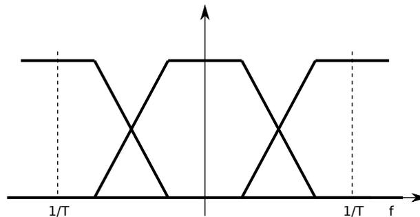
Figure 2: Superposition of shifted versions of  $G_{\text{TX}}(f)$
