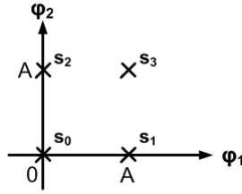
Figure 1: Signal Constellation for  $\bar{x}_{bb}$
