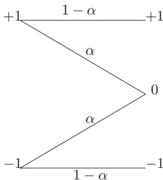
Figure 2: Binary erasure channel with erasure probability  $\alpha$
