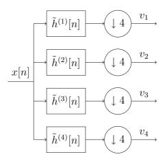
Figure 7: Equivalent filter bank with constant downsampling rate
