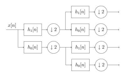
Figure 6: Tree structured filterbank
