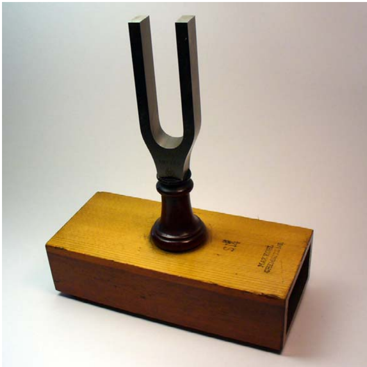
Tuning fork on resonance box
