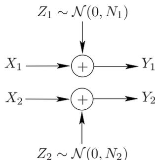
Figure 1: Parallel Gaussian channels
