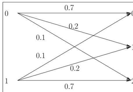
Figure 3: Symmetric channel with 2 inputs and 3 outputs
