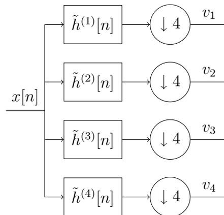
Figure 7: Equivalent filter bank with constant downsampling rate
