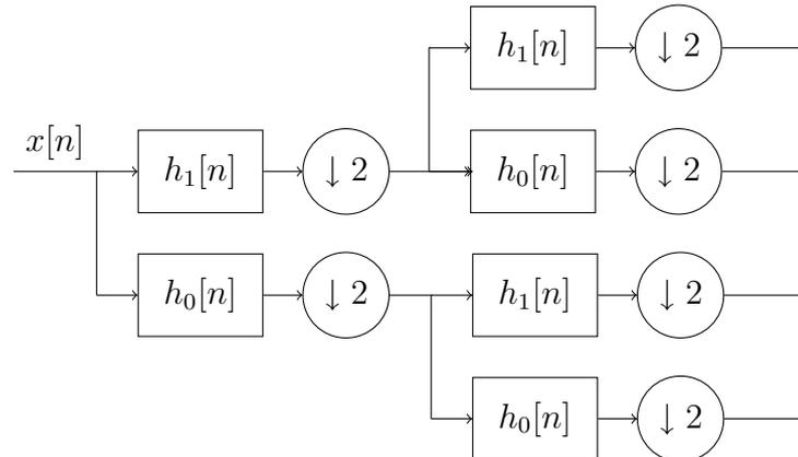
Figure 6: Tree structured filterbank
