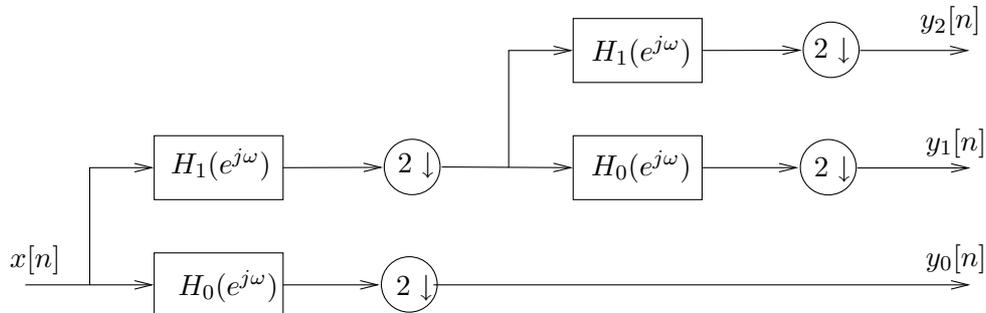
Figure 6: Tree-structured Analysis filter bank
