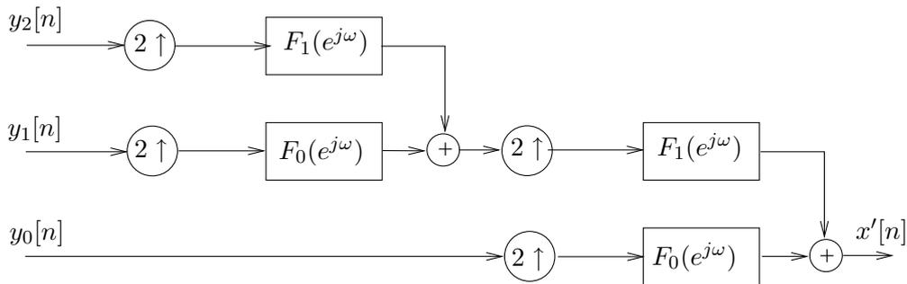
Figure 9: Tree-structured synthesis filter bank
