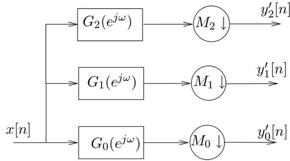
Figure 8: Equivalent Analysis filter bank
