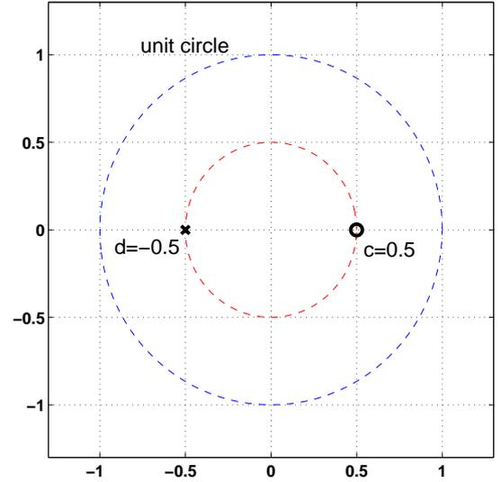
Fig. 3: The zero-pole plot of  $H(z)$  for  $\phi = \pi$ .
