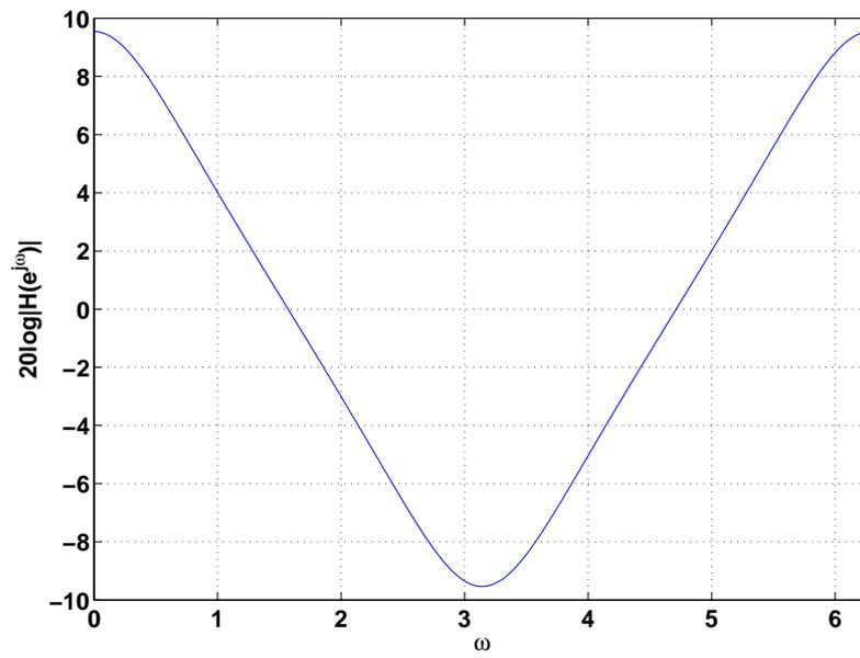
Figure 4:  $20 \log_{10} |H(e^{j\omega})|$  for  $\phi = 0$ .
