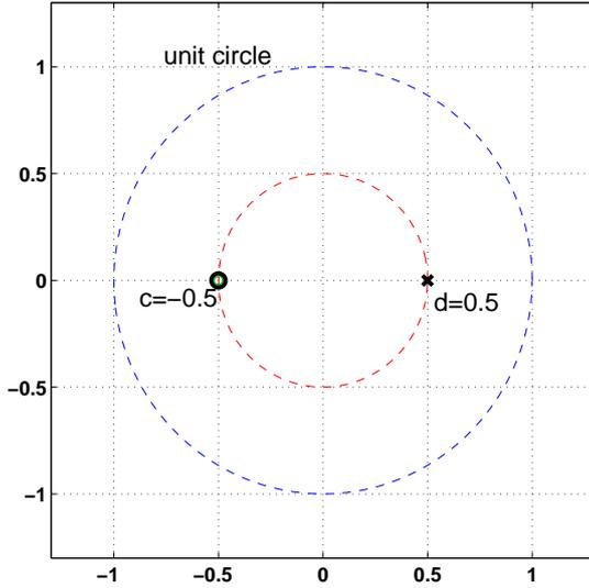
Fig. 2: The zero-pole plot of  $H(z)$  for  $\phi = 0$ .
