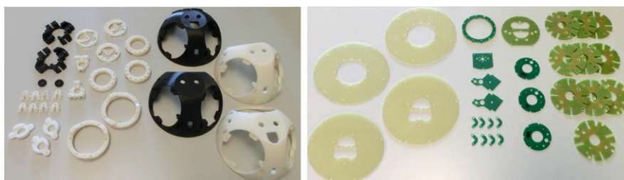
Fig. A.21. Left: Printed elements of one Roombots module. 52% (volume) of RB components are 3D printed from ABS material. Right: glass fiber sheet material used in Roombots.
