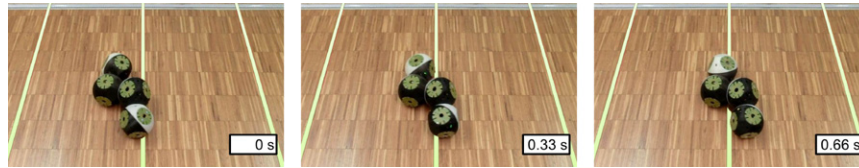
Fig. 11. First off-grid Roombots metamodule (MM) locomotion type: MMs use the module's outer spheres as wheels, only two of six joints are active. The distance between light-green marker lines is 0.5 m. The maximum continuous locomotion speed was 13 cm/s, and the direction of locomotion is to the right. Marker lines on the floor were emphasized to identify module movement. (For interpretation of the references to colour in this figure legend, the reader is referred to the web version of this article.)
