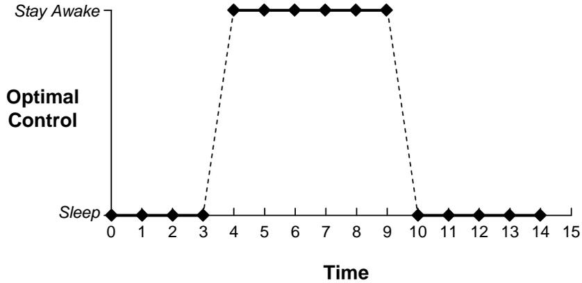
Fig. 3. Optimal control policy at  $X_k = \begin{bmatrix} 0 \\ 0 \end{bmatrix}$  when  $T = 15$ ,  $N = 3$ ,  $c = 10$ ,  $D = 21$ , and  $p = \frac{2}{3}$
