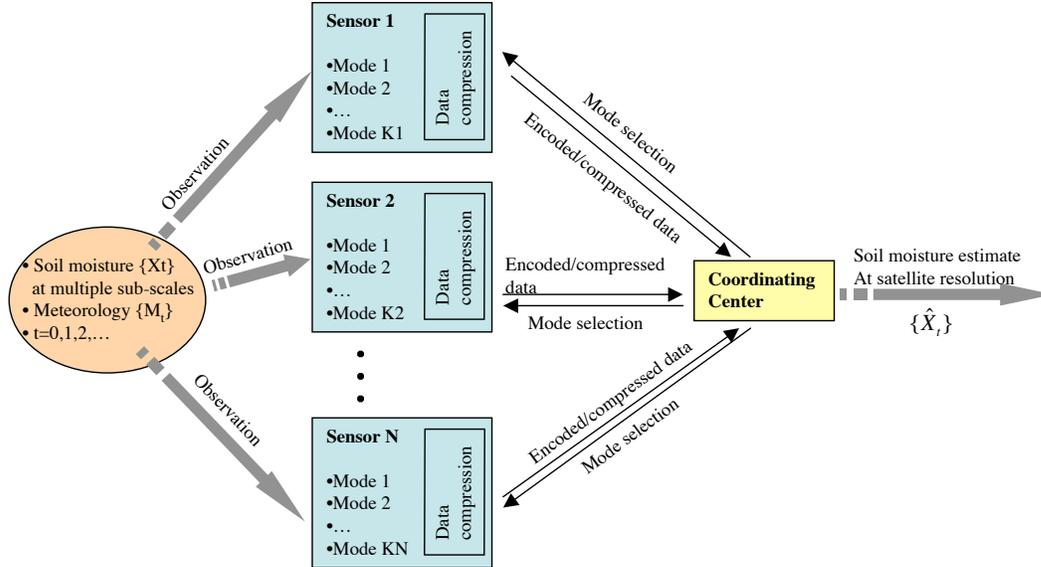
**Figure 2.** Control architecture. Each sensor measures variables over a finite period of time. Variables are correlated with the soil moisture field. Data are compressed at each sensor node and transmitted to the coordinating center, which derives an optimal control instruction set for the sensors, as well as an unbiased estimate of the soil moisture field at the remote sensor resolution, guided by data assimilation.
