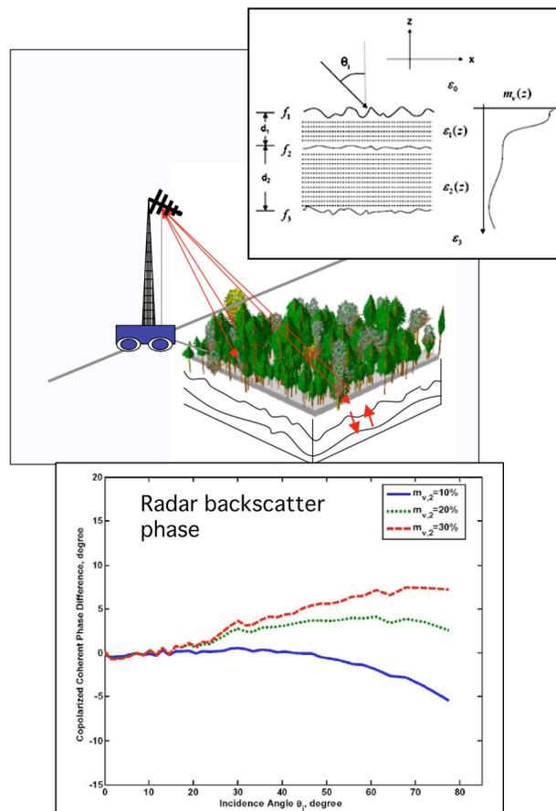
Figure 5. Top: a realistic soil moisture profile from surface to a depth of  $d_1+d_2$ . Middle: remote sensor could be a low-frequency radar (tower-mounted, airborne, or spaceborne) which can produce measurements related to soil moisture profiles at varying depths. Bottom: Example of backscattered co-pol phase dependence on moisture profile, to be used in developing inversion algorithms.
