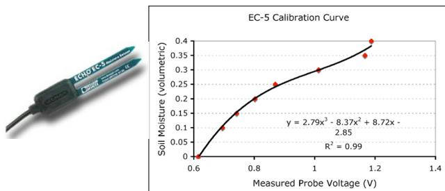
Figure 4. Left: the Decagon ECH<sub>2</sub>O EC-5 soil moisture probe. Right: calibration curve (or “sensor model”) derived from experimental data and used in the control algorithm.
