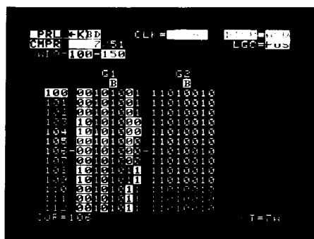
You can compare the data you have just acquired to a set of data in reference memory. All differences are displayed in reverse video.
