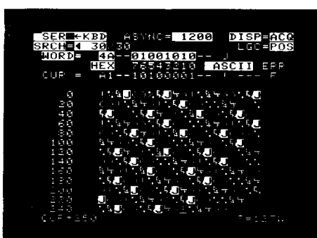
Captured serial data can be displayed in state or character format. Data can also be searched for occurrences of a specified word.
