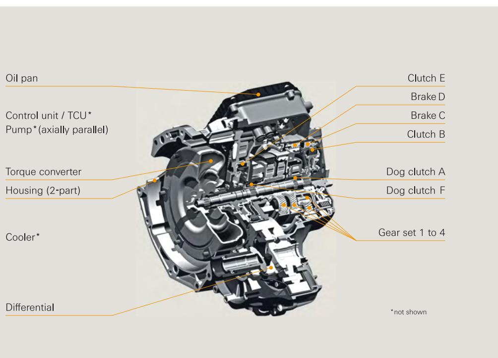
Extremely compact package dimensions (length x depth x height = 367 mm x 621 mm x 428 mm) and an astonishingly low weight of 86 kg (189 lbs.) including oil (9HP48).
