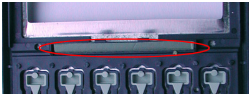
Rubber Under Keyboard Contacts
