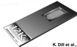
Mounted chip (on PCB) and sensor site from 1k Combinatrix array using conventional optical readout.
