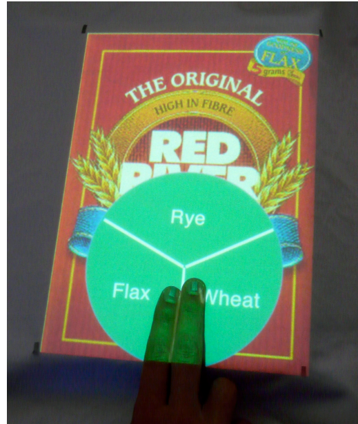
Figure 1. Cloth draped over a cereal box provides an interactive menu to its ingredients in a language of choice.
