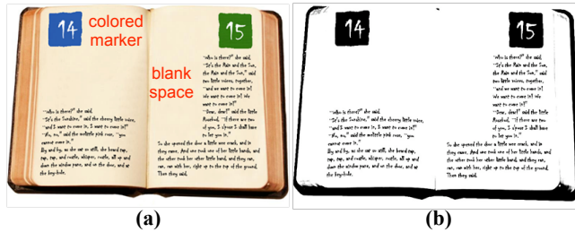
Figure 3. Page layout; a) colored markers and blank space on pages; b) binarized image of what the camera sees with the colored markers converted to black
