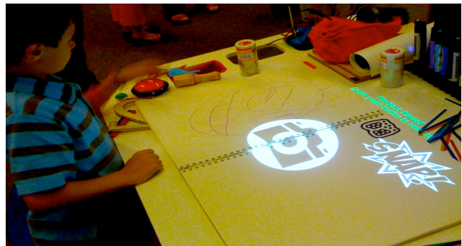
Figure 3. Child presses the red “capture” button to save and send a snapshot of his drawing to other creation-stations, corresponding to the correct page with the same Fiducial marker.
