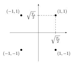
The mapping is such that neighboring points differ by one bit. This minimizes the biterror probability since when we make an error chances are that we choose a neighbor of the correct symbol. Notice that we may decode each bit independently. In fact the first bit is decoded to a 1 iff the observation is to the right of the vertical axis and the second bit is 1 iff it is above the horizontal axis. The bit error probability is therefore
