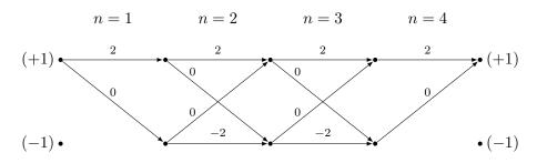
(ii) The Viterbi algorithm uses the path metric  $|S[n] - (I[n] + I[n-1])|^2$  and finds the path with smallest metric (closest path to the output sequence) on the trellis. Given the output sequence (2, -1, 0, 1) the edges will be labeled as follows:
